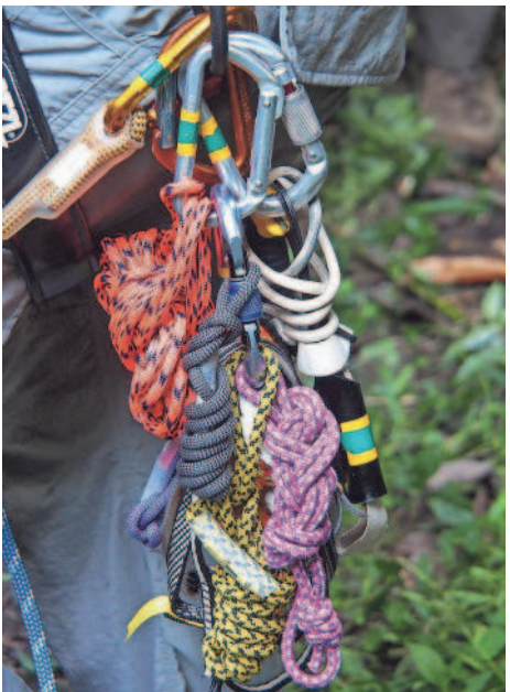
Search and rescue team members wear climbing harnesses bearing brightly colored bundles of rope slings and clusters of metal climbing devices on the side loops of their harnesses.
